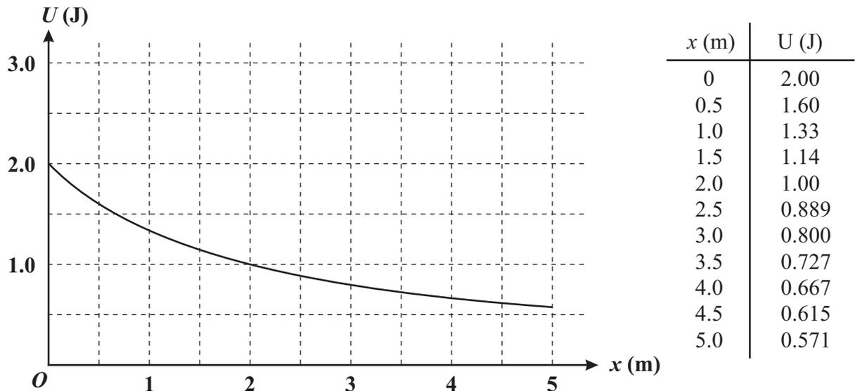
(b) By definition,  $U = Fx$ , so  $F$  can be found by taking the slope of the  $U(x)$  versus  $x$  graph which is accomplished by differentiating  $U(x)$  with respect to  $x$ .  $U(x)$  can be written as  $4.0(2.0 + x)^{-1}$ .
