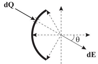
$$(c) V = k \frac{Q}{R} = \left( 9.0 \times 10^9 \text{ N} \frac{\text{m}^2}{\text{C}^2} \right) \frac{(\pi \times 10^{-6} \text{ C})}{0.10 \text{ m}}$$
